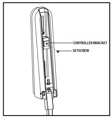
Figure 16. Underside of Armrest
